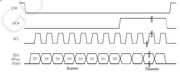
Figure 3.5-1: Write procedure in 4-wire SPI mode
