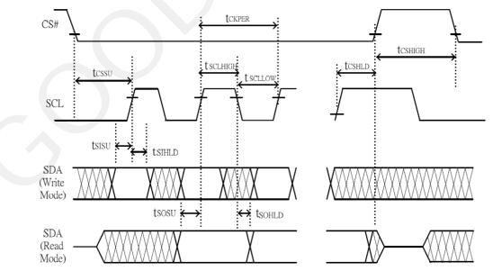
Figure 3.3-1: SPI timing diagram
