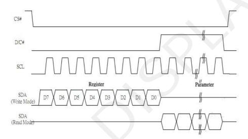
Figure 3.5-2: Read procedure in 4-wire SPI mode
