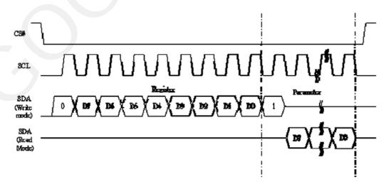
Figure 3.5-4 Read procedure in 3-wire SPI mode
