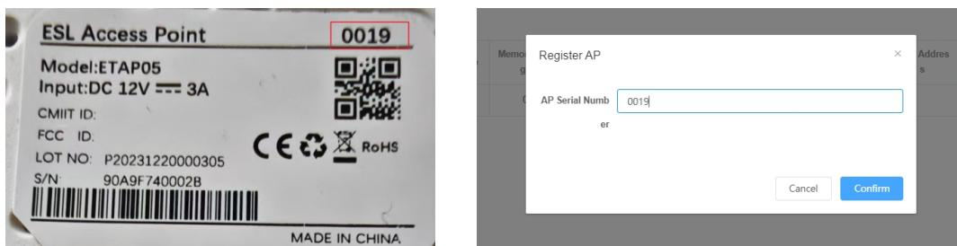
Connect the AP to the power supply and connect the network cable to the port of the router. The AP status is displayed online and registration is complete.
